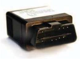
DriverPoint Telematics device's "plug in and go" installation
